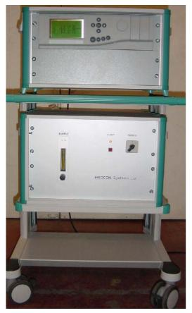
The model MOD-1002 Mobile Emissions Monitor is easily transported system, designed to provide affordable state-of-the-art accuracy, stability and reliability. The system comprises an infrared / paramagnetic analyzers and advanced sample conditioning assembly to produce accurate and reliable measurement of four components simultaneously: O2, CO, NO, CO2.
