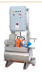
The Sample Recovery System offered by Modcon designed to collect spent sample from on-line process analyzers and periodically return this sample back to the process lines
